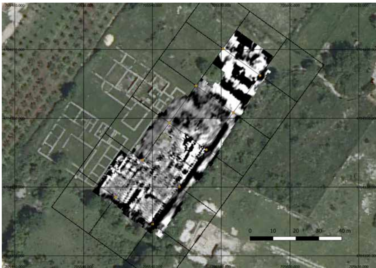
Fig. 2 - Results of the earth resistance survey in the east part of the site over orthophoto of the site. Figure by Tomasz Dziurdzik and Michał Pisz.
